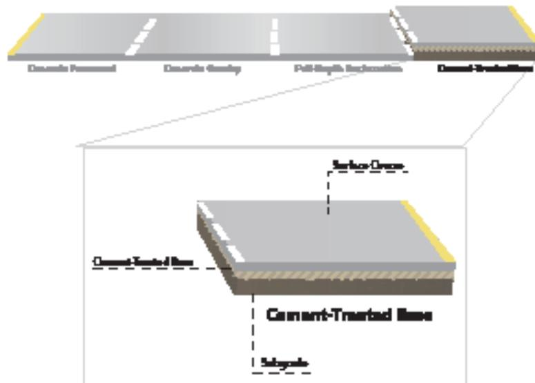
Without a solid base, roads don't stay roads for long. A weak base leads to the rutting, alligator cracking, and potholes commonly associated with asphalt. Cement-treated base gives your road surface a solid backbone that spreads loads across a wider area, minimizing the impact of traffic and making your investment last years longer. To learn more, visit [www.think-harder.org/paving](http://www.think-harder.org/paving).
