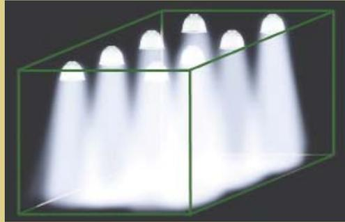
Not all lighting fixtures are created equal. Inferior optic design can actually require more fixtures and provide less uniform illumination (top). Optimized optical control can dramatically improve distribution and uniformity, with fewer lighting fixtures (bottom).
