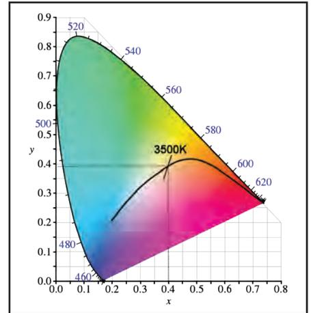
These bins are grouped as quadrants around the standard chromaticity lines (shown below in blue) for a specified color temperature. The larger the bin size, the more variation around the standard color temperature is accepted. Conversely, smaller bin sizes maintain a tighter control of color variation.
